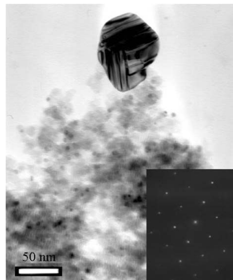
Fig. 4 TEM image of silica aerogel matrix impregnated with complex [A] and corresponding diffraction pattern (111 plane of metallic silver).
